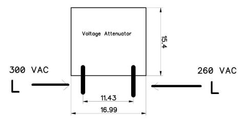
All Dimension are in mm Hole Dimension is 1 mm.
